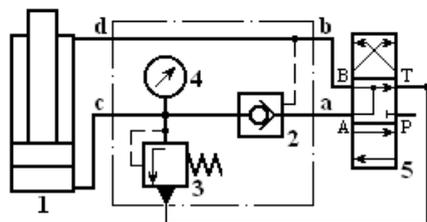
Fig. 1. Hydraulic prop: basic structure
