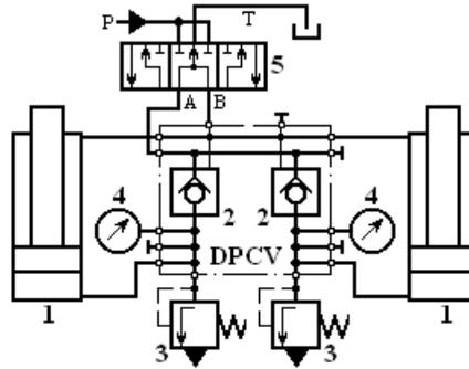
Fig. 2. Basic hydraulic diagram of props from a shield of a powered roof support
