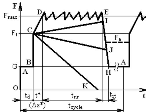
Fig. 3. The operation of hydraulic props
